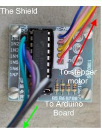
Plug the stepper motor harness into the shield. It only fits one way round.
